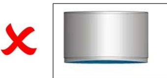
**Figure 13** Pot base is bowed inward and is **NOT FLAT**; The unit efficiency will be dramatically reduced during cooking. It may not even be detected by the appliance.
