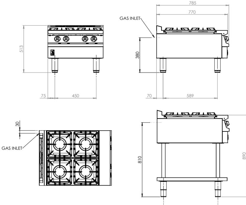
Measurements *in mm* Unit on castors is the same hob height
