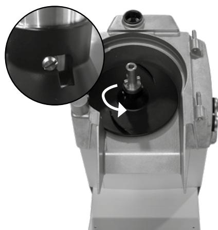
FITTING THE EJECTOR PLATE
