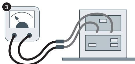
High voltages and large currents are present at the High Voltage Capacitor. It is very dangerous to work near this part when the oven is on. NEVER make any voltage measurements at the High Voltage circuits, including the magnetron filament.
