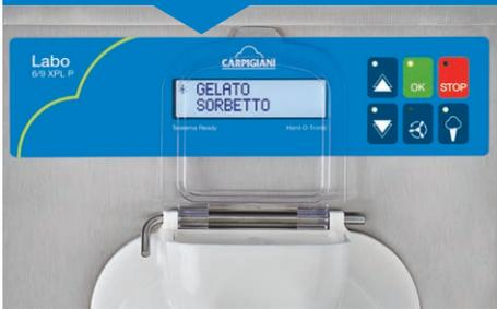
When the hopper lid is open **all the command buttons are still fully accessible**, allowing you to start the production cycles even while adding the ingredients.
