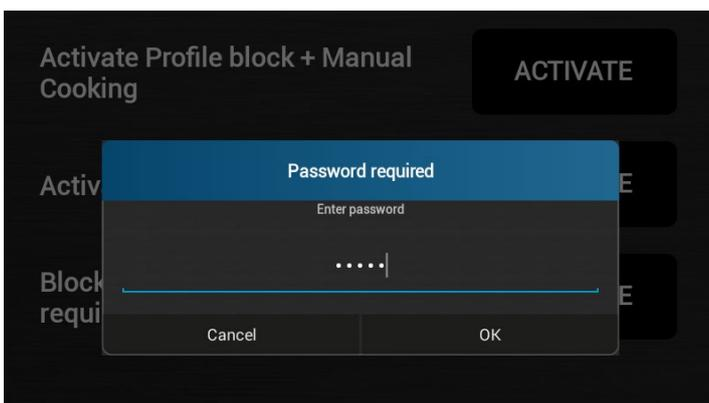
To activate the chosen block, press **“ACTIVATE”**, then enter the password and repeat it to confirm.
