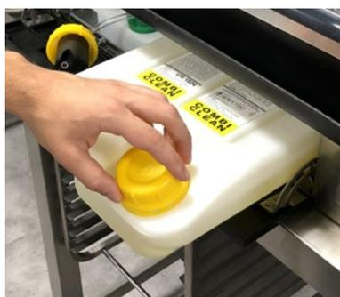
Remove the top of the new cartridge.
