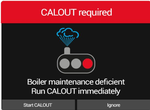
If **CALOUT** is not performed, once the maximum maintenance interval is reached, the following popup appears: **“Boiler maintenance needed, perform CALOUT immediately.”**
