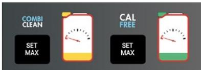
On the oven display, press the “**SET MAX**” key which corresponds to the **COMBICLEAN** or **CALFREE** that has been replaced.
