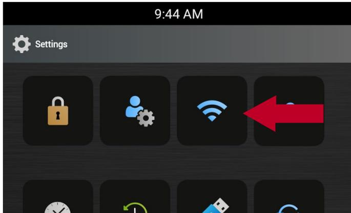
Press the icon “**Wi-Fi Settings**” to check the activation and availability of the Wi-Fi connection.
