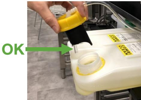
Insert the cap with the extraction system (**YELLOW** for **COMBICLEAN** detergent and **GREEN** for **CALFREE** descaler) ensuring that the clear extraction pipe is facing the front of the cartridge as shown in the figure.
