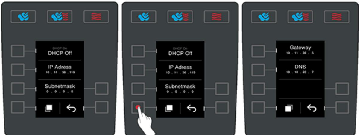
The DHCP number, IP address, subnet mask, gateway and DNS are displayed here. The MAC address is also displayed here. For example, in a company environment, the network connection can be assigned by the unique identifier of the network adapter of the iCombi Classic (MAC address).
