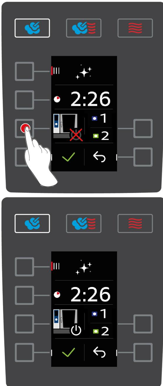
The "automatic switch off after cleaning end" function is now activated.
